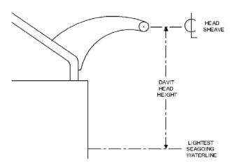
Figure P-2: Representation of davit head height for calculating lowering speed
