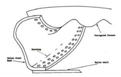
Grooving in this area, when it is not extensive, may be repaired by chipping out the groove to sounds metal, non-dextructive testing and subsequent welding. Extensive grooving, or fractures stemming from old grooving previously welded can be repaired only by cutting gout and renewing a portion of the head plating.
