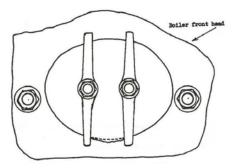
Repair consists of thorough cleaning or grinding to sound metal, magnetic particle testing to ensure no fractures exist and building up of original thickeness by welding.
